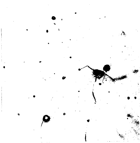
Fig. 55 50% Niobium. (Annealed 40 hours at 1075°C. Made with niobium sheet. 2:1:1:1:HNO 3 :H 2 SO 4 :HF:H 2 O etch. X250).
