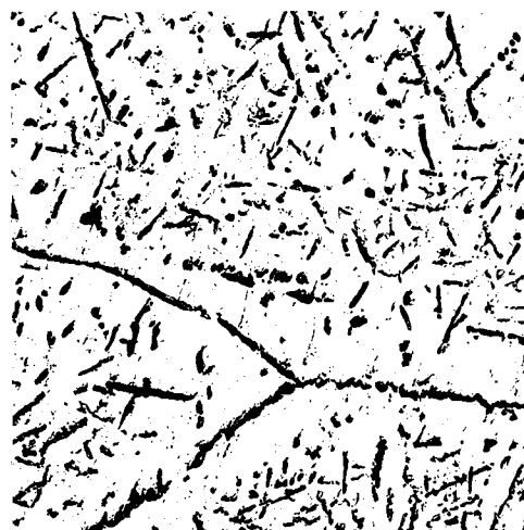
Fig. 31 Niobium. (As arc melted. Grain boundary material and needles are impurities. Aqua regia plus 5% HF etch. X250).
