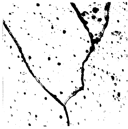
Fig. 56 30% Niobium. (Annealed 40 hours at 1075°C. Made with niobium sheet. Same etch. X250).
