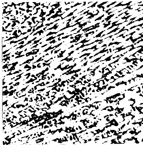
Fig. 28 72% Niobium. (As arc melted. Niobium dendrites and eutectic. Electrolytic etch. X100).
