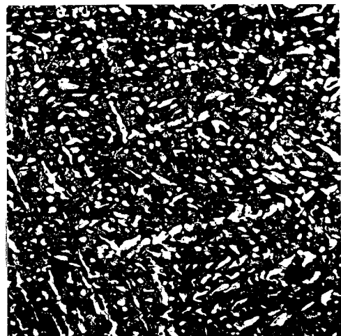
Fig. 17 25.5% Niobium (Annealed at 1285°C., furnace cooled. Niobium plus eutectic. Electrolytic etch. X250).
