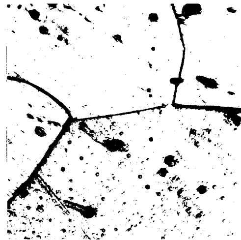
Fig. 46 20% Niobium. (As arc melted. Made with niobium powder. Same etch. X250).
